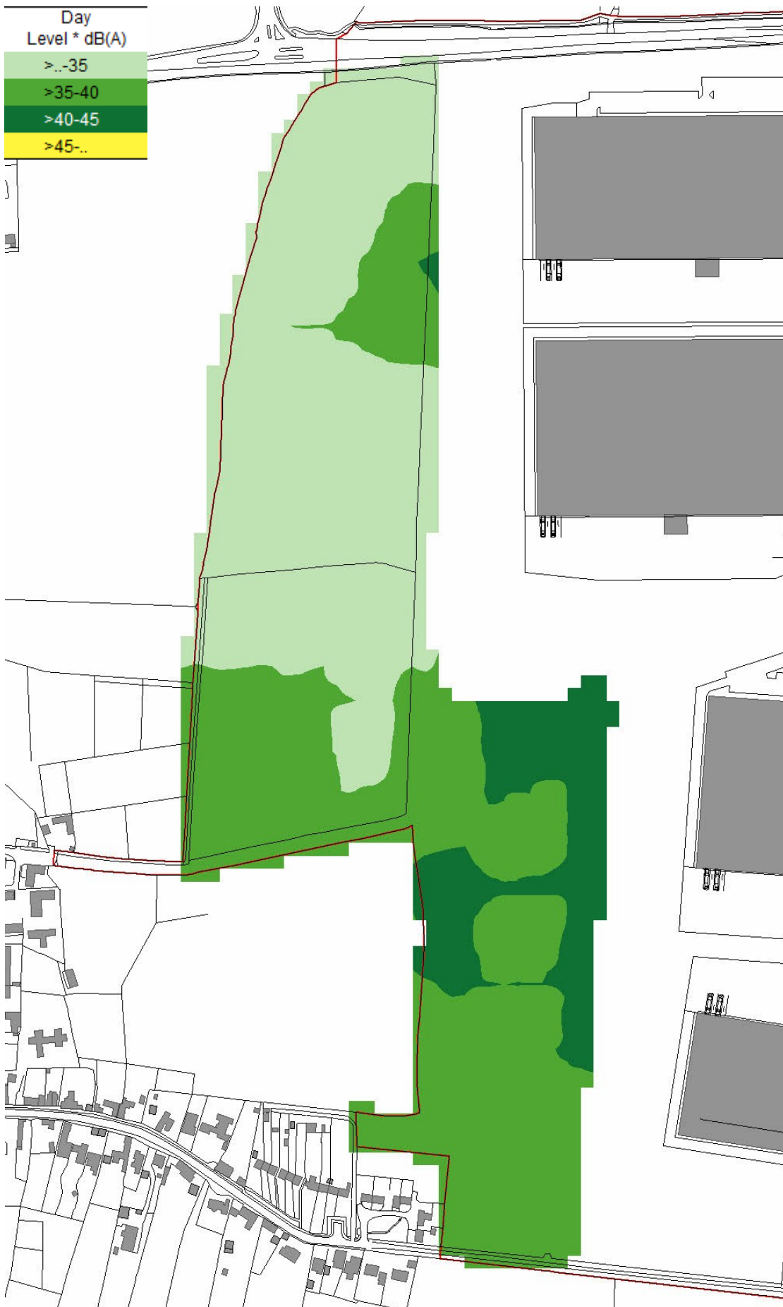
Figure 2—1: Predicted operational sound levels from EMG2 Main site during worst-case 1-hour period of day (dB L_{Aeq,1hr} , illustrative landscape masterplan layout)
