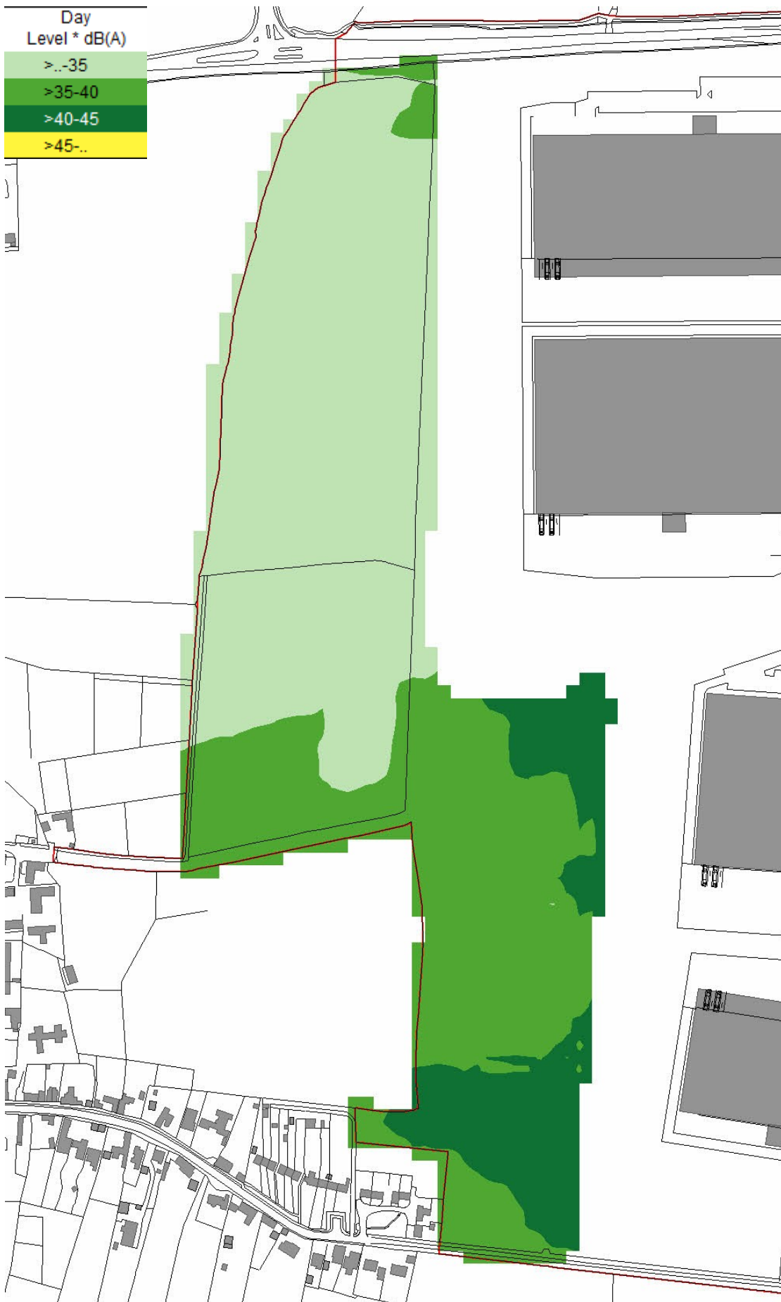
Figure 2—2: Predicted operational sound levels from EMG2 Main site during worst-case 1-hour period of day (dB L_{Aeq,1hr} , alternate layout)
